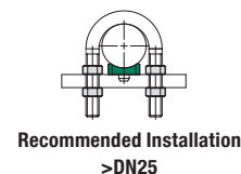
Round Steel U-Bolt (type RB) with Plastic Pipe Saddle (type RUK)
