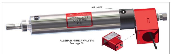
Cylinders are available with 1-1/8" bore only. They are Single Acting Cylinders controlled by a 3-way Single Solenoid Valve mounted to the rear head of the units. The standard solenoid operator (as shown) is the **AAS** splice box housing. A general purpose conduit housing **(AAC)** is also available. Most common AC & DC voltages are available. 12, 24, 120 & 240/60 and 6, 12 & 24/DC are standard. The basic construction is the same as our 1-1/8" bore Type "A" Cylinders.
